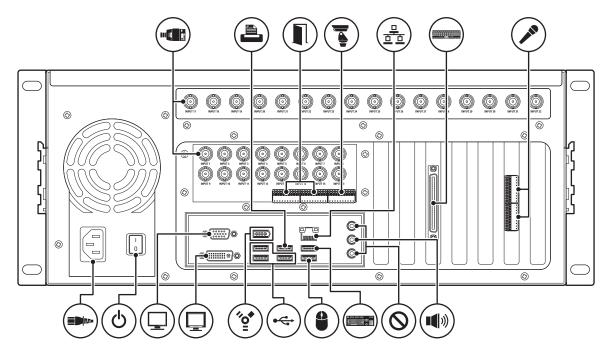
**NOTE:** The top row of video input BNCs (inputs17-32) is available only on 32-input systems. The SCSI connector for RAID storage is optional.
